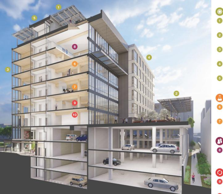
**Rooftop Solar - PV Array** Annual production 436 MWh of energy - Zero Net Energy use for APEX offices. Solar Array - PV Canopy PV Canopy provides shade cover and renewable energy. High Performance Glazing Thermally broken window frame, SOLARBAN 90 insulated glazing unit. **High Performance Opaque Envelope** Cross-laminated timber, DensElement<sup>™</sup> weather barrier, Thermafiber rigid insulation, thermally broken rainscreen structure, rainscreen cladding.
